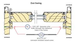
E. Drill 13/64" clearance holes through the threshold but not into the rough opening, at the locations shown in illustration on previous page (5E & 5G). Install # 10 x 3/1-2" corrosion resistant wood screws through the threshold into the floor. For Masonry applications use masonry screws that are a minimum size of 3/16" diameter x 3" and pilot drill per screw manufacturers's recommendations.
